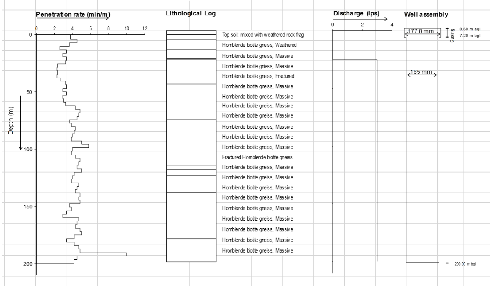
Fig. 2(a) Drill time log, Lithological log, Discharge and Well assembly of the borehole drilled at NELLIPUZHA O/W
