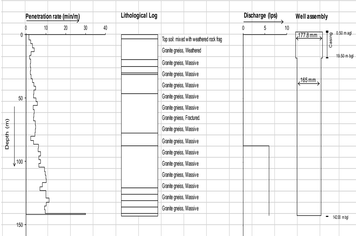
Fig. 2 Drill time log, Lithological log, Discharge and Well assembly of the borehole drilled at BHIMANAD E/W
