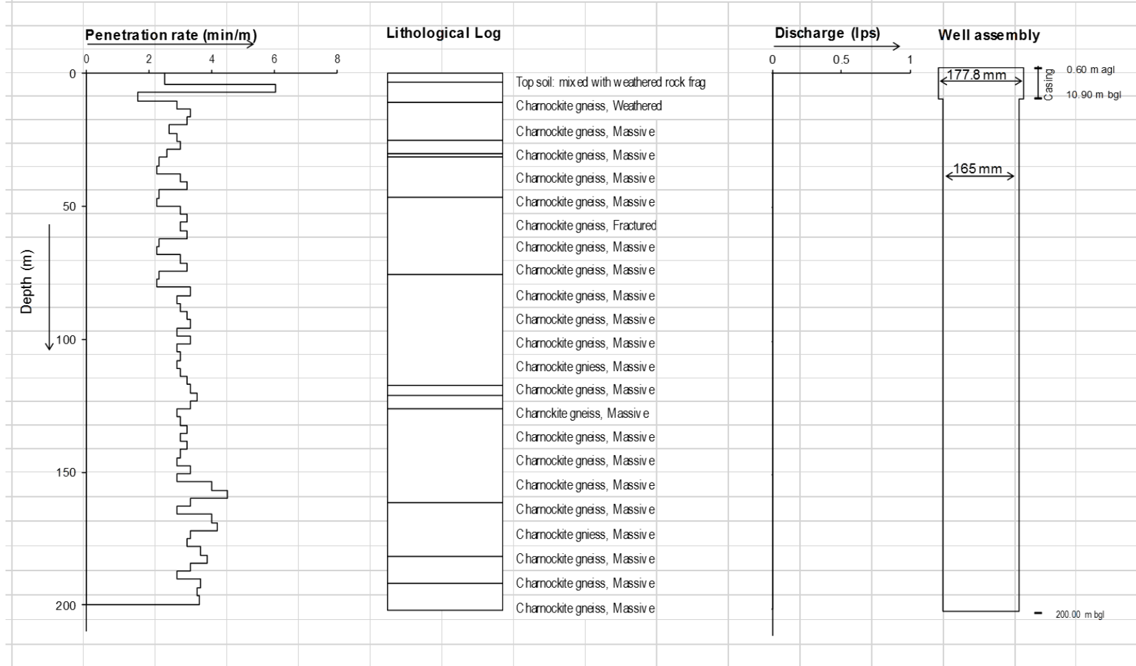
Fig. 2 Drill time log, Lithological log, Discharge and Well assembly of the borehole drilled at THIRUVIZHAMKUNNU E/W
